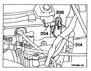
4 Push relay lever (214) to full throttle; this must cause the injection pump control lever to move against the full throttle stop (arrow) and the roller (215) to be positioned approx. 1 mm before the end stop in the gate.
