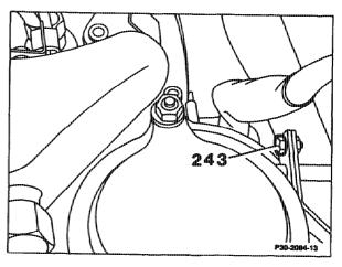
1st version Full throttle adjusting screw (243) on the accelerator control shaft
