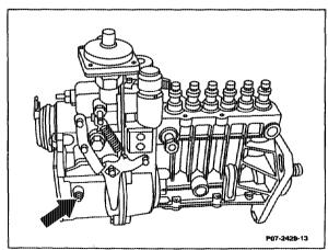
If not, slide the adjustable ball head (206) in the elongated hole of the relay lever.
