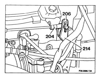
4 Pull accelerator control lever (208) to full throttle; this must cause the roller (215) to be positioned approx. 1 mm before the end stop in the gate and the injection pump control lever to move against the full load stop (arrow).
