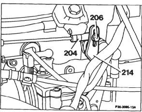
4 Pull accelerator control lever (208) to full load; this must cause the roller (215) to be positioned approx. 1 mm before the end stop in the gate and the injection pump control lever to move against the full load stop (arrow).
