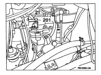
6 Adjust control pressure cable. Press off ball socket (212) for this step. Pull control cable forward until a slight resistance is felt. In this position, attach ball socket free of tension. Adjust Bowden cable (211), if necessary.
