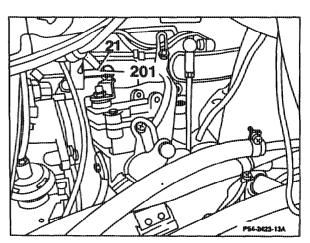
6 Adjust control thrust cable. Press off ball socket (212) for this step. Pull control cable forward until a slight resistance is felt. In this position, attach ball socket free of tension. Adjust Bowden cable (211), if necessary.
