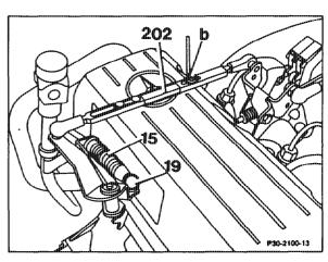
8 Check full throttle stop, adjust. With the engine switched off, depress accelerator pedal fully to the stop on the kickdown switch from the interior of the car. This must cause the control lever to move against the full load stop (arrow) of the injection pump.
