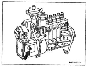
5 Adjust, if necessary, at adjustable ball head (206) in the elongated hole of the relay lever.
