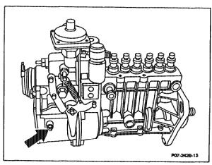
Slide the adjustable ball head (206) in the oblong hole of the relay lever (214), if necessary.
