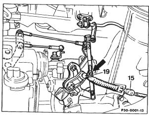
2nd version Full throttle adjusting screw on the connecting rod (203)
