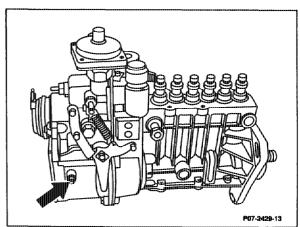
Adjust at the adjusting screw (229), if necessary.
