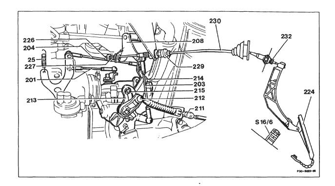
Accelerator control linkage examine for bending and ease of movement.
