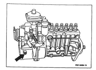
Adjust at the adjusting screw (243), if necessary.
