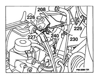
Adjust Bowden cable (230), if necessary, with the adjusting nut (232) from the interior of the car.
