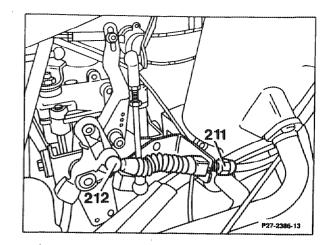
7 Check full throttle stop, adjust. With the engine switched off, depress accelerator pedal fully to the stop on the kickdown switch from the interior of the car. This must cause the control lever (arrow) to move against the full load stop of the injection pump.
