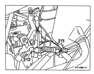
7 Check full throttle stop, adjust. With the engine switched off, depress accelerator pedal fully to the stop on the kickdown switch from the interior of the car. This must cause the control lever (arrow) to move against the full load stop of the injection pump.
