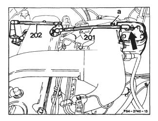
7 Adjust control push cable. Press off ball socket (212) for this step. Pull control cable (211) forward until a resistance is felt. In this position, attach ball socket free of tension. Adjust at the hexagon bolt (b), if necessary (measure connecting rod (202) pulled out).
