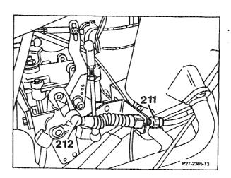
7 Check full throttle stop, adjust. With the engine switched off, depress accelerator pedal fully to the stop on the kickdown switch from the interior of the car. This must cause the control lever to move against the full throttle stop (arrow) of the injection pump.
