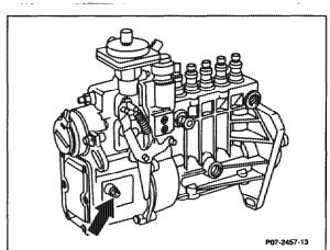
Adjust Bowden cable at adjusting screw (229), if necessary.
