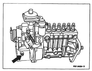
Adjust at the adjusting screw (229), if necessary.
