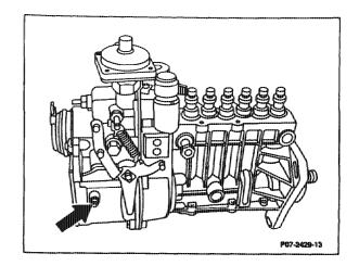
Slide the adjustable ball head (206) in the elongated hole of the relay lever (214), if necessary.
