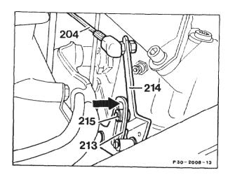
4 Pull accelerator control lever (208) to full load; this must cause the injection pump control lever to move against full load stop (arrow) and the roller (215) to rest approx. 1 mm before the end stop in the gate.
