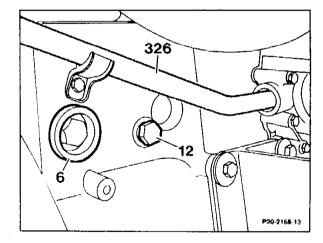
Engine 601 12 Drain plug on crankcase
