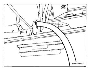
Extension hose fitted on (with air conditioning)
