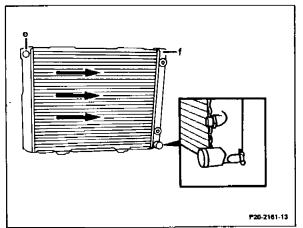
Drain plug on models with air conditioning
