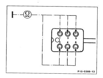
If  $\infty$   $\Omega$  resistance is measured, there is an interruption of the respective glow plug or of the lead or of the connection. Rectify interruption in the lead or renew glow plug.
