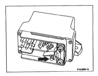
If no voltage is indicated, test red cable from starter, terminal 30, to the preglow time relay, terminal 30, for interruption. Rectify interruption.
