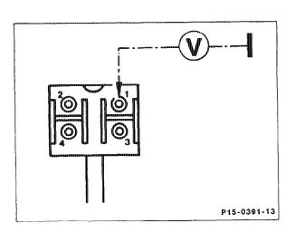
If voltage is indicated when preglow system is switched on, test pink/red cable from fuse 7 (unprotected side) through plug connection of engine wiring harness to contact 1 of the connector of the preglow time relay for interruption. Rectify interruption.
