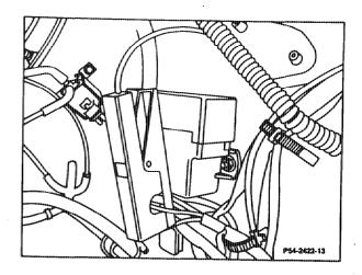
Detach the 6-pin connector from the preglow time relay to test for interruption.
