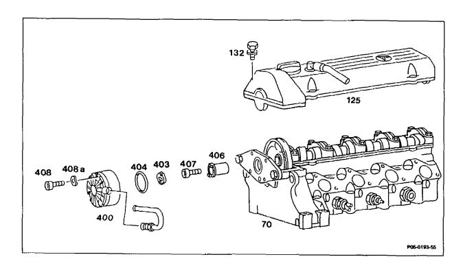
Cylinder head cover (125) ..... remove, install, fastening bolt (132), 10 Nm. Pressure oil pump (400) ...... unscrew, screw on, fastening bolt (408) with washers (408a), 11 Nm, put pressure oil pump to one side with lines connected.
