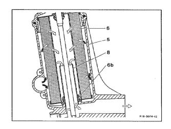
The oil filter housing is supplied in the parts sector only as a running-in oil filter which in this case should be replaced with the normal oil filter element.
