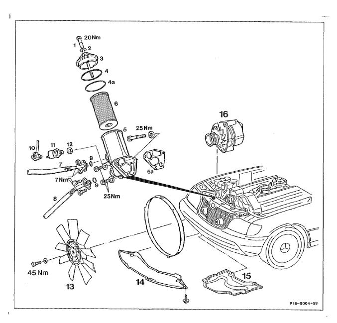
Engine compartment panel ...... remove, install.
