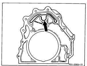
6 Coat radial seal between dust and sealing lip with engine oil.
