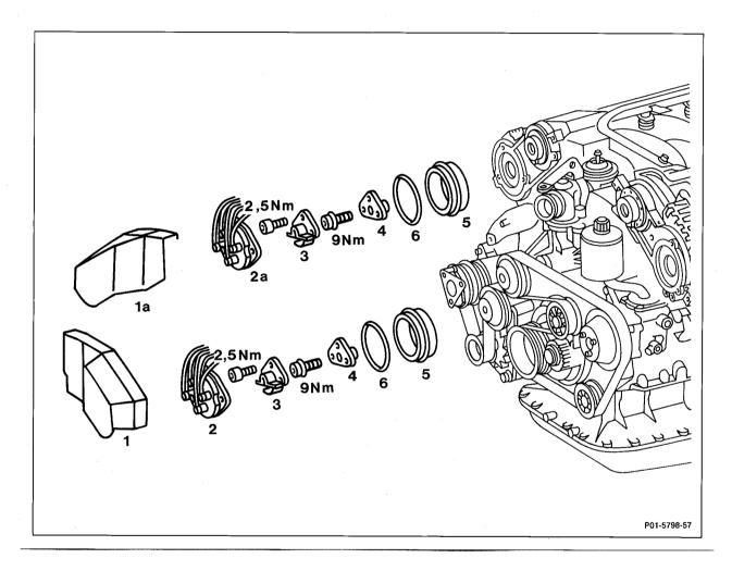
Shielding caps (1) and (1a) at the side ...... unclip, take off, fit on.
