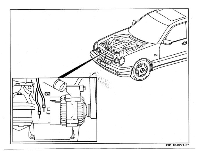
Wiring at generator (G2) ..... unbolt, bolt on.
