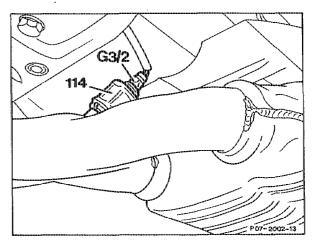
Oxygen sensor plug connection (G3/2x1) .....
