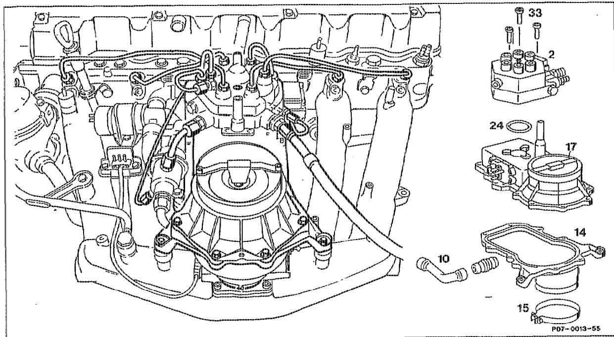
Fuel distributor (2) ..... unscrew from air flow sensor (17), screw on
