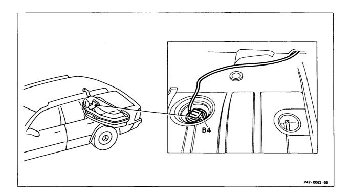
Battery ground cable ..... disconnect, connect. Front load area flap or 3rd bench seat back remove, install. rest ...... partially remove, install. Load area trim ....... Cover ....... unclip, clip in place. Coupling at fuel gauge sender (B4) ..... unplug, plug in. Fuel gauge sender (B4) ..... remove, run empty if necessary, install. Replace seal. Remove securing pin below adhesive strip (only new part). Tightening torque 40 Nm.
