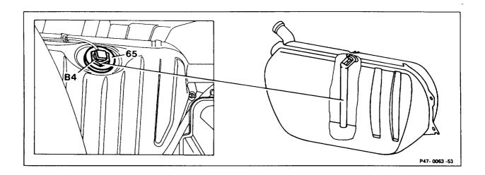
Battery ground cable ...... disconnect, connect. Fuel tank trim ..... remove, install.
