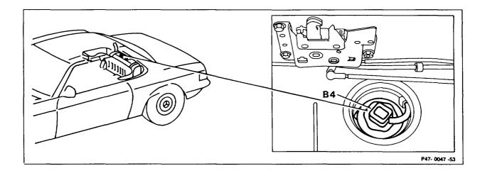
Battery ground cable ..... disconnect, connect. Hardtop ..... take off, fit on. Soft top ..... open, close. Cover ..... unclip, clip in place. Coupling at fuel gauge sender (B4) ...... unplug, secure against slipping off, plug in. Fuel gauge sender (B4) ..... remove, run empty if necessary, install. Replace seal. Remove securing pin below adhesive strip (of new part). Tightening torque 40 Nm.
