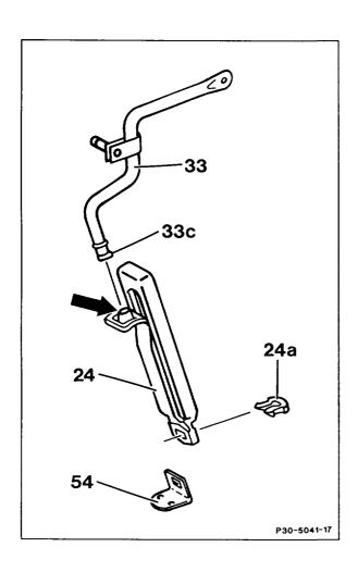
Lugs of expanding clip (24a) . . . . . . . . . . compress behind accelerator pedal (24).
