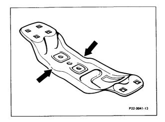
Thickness of engine carrier material, production breakpoint: 08/1987
