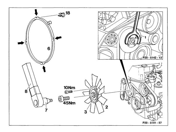
Locking pin (18) ..... remove, insert.
