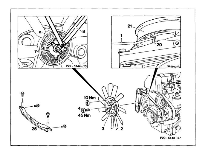
Screw (4) of viscous fan clutch (3) ......
