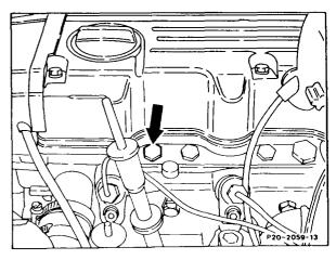
6 If car fitted with auxiliary heater: Take off cap (635), unscrew bleeder screw (636) slightly until no more air flows out.
