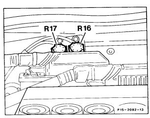
R16 EZL resistance trimming plug R17 KE resistance trimming plug
