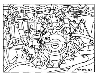
3 Screw shop-made fuel hose onto diaphragm pressure regulator and hold in measuring glass or beaker.
