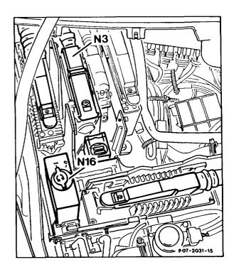
N3 KE control unit N16 Engine systems control unit
