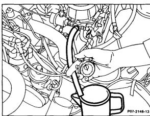
4 Bridge contacts 7 and 8 at fuel pump relays (N16/1 to N16/4), on model 129 engine systems control unit MAS between contacts 1 and 2, for
