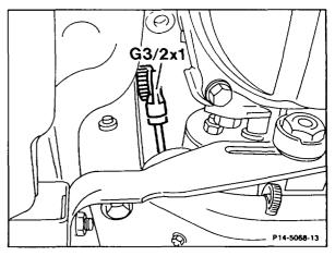
Model 129 G3/2x1 Plug connection, oxygen sensor
