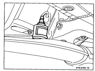
Cable of oxygen sensor with rubber grommet ...
