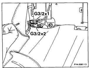
G3/2×1 Plug connection, oxygen sensor heating coil G3/2×2 Plug connection, oxygen sensor signal
