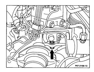
When detaching the fuel line (50) from the fuel distributor to the diaphragm pressure regulator, ensure that the open-end wrench does not press onto the air flow sensor position indicator and damage it.
