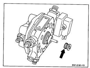
Position (arrow) of screw plug measure with depth gauge and note. As a precaution, mark position with marking tool.
