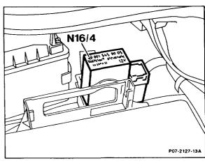
7 Bridge the two contacts 7 and 8, on model 129 engine systems control unit MAS between contacts 1 and 2, for (SA) J as of model year 1990 on KE control unit (N3) between contacts 11 and 20. This causes the fuel pump to be energized.
