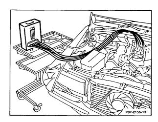
4 Connect lines of fuel quantity measuring instrument to fuel distributor (see Fig for sequence) and place fuel return line into the filler neck of the fuel tank.
