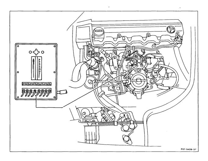
Fuel quantity comparison instrument .... position on level point next to vehicle.
