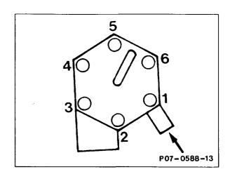
5 Clamp adjusting device for fixing position of air flow senser plate to stop bar of air funnel.
