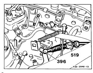
13 Models 107, 126: press off accelerator control linkage (arrows) and turn to the left and tie tight.
