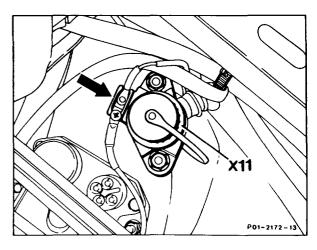
18 Unscrew bolts (arrows) for exhaust system at the flange of the exhaust manifold.
