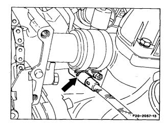
8 Slacken hose clip (235). Detach heating water return line (236).
