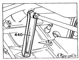
7 Slacken hose clips (arrow) at coolant hose to coolant pump.
