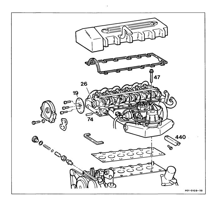
Camshaft sprocket (19) . . . . . . . . . mark relative to camshaft (26), detach and
