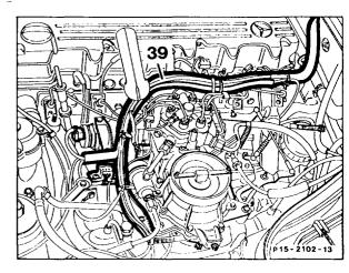
16 Detach control cable and vacuum line at the connector-sensor ignition control unit.
