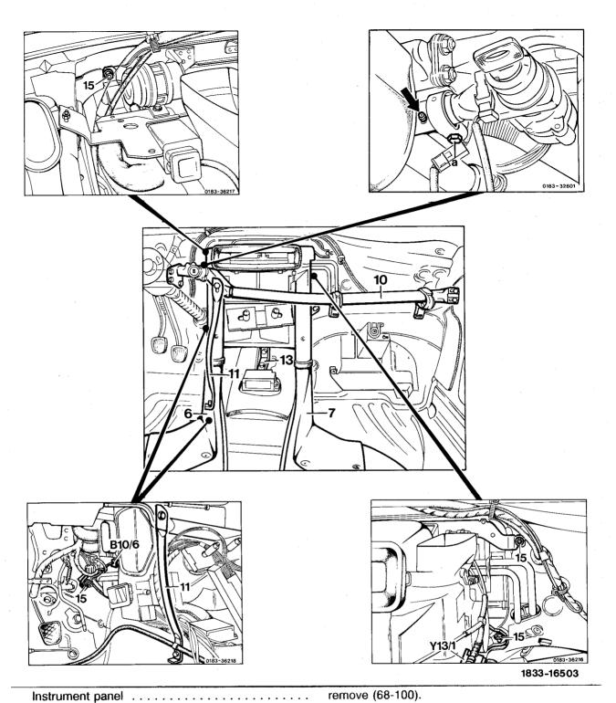
2-pole connector on left and right heat exchanger temperature sensors (B10/2 and B10/3) and evaporator temperature sensor (B10/6) ......
