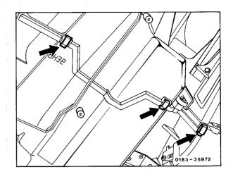
11 Unclip three clamps each on right and left sides of heater and air conditioner box and one clamp in the center (arrow).
