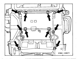
2 Unscrew4 screws (17) and remove cover (19).
