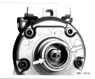
5 Position key puller on compressor shaft and turn one half turn to right.
