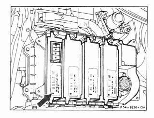
The individual connection fields in the module box are identified by number. This, along with the color-coded connectors, allows easy coordination of the wiring harness with the respective connection field and control unit.
