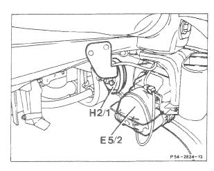
E5/2 Right fog lamp H2/1 Fanfare horn 2 The ellipsoid fog lamps are installed below the front bumper in the spoiler area.
