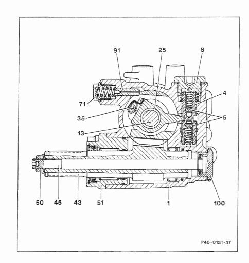
4 Control valve Reaction piston 8 Cover 13 Steering worm 25 Steering nut 35 Steel balls 43 Pitman shaft Adjusting screw Self-locking collar nut Housing cover 45 50
