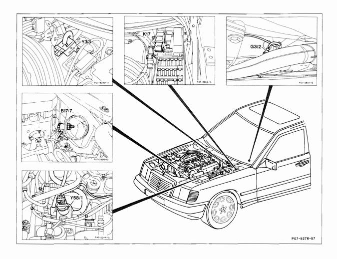
B17/7 G3/2 K17 Intake air temperature sensor Heated O<sub>2</sub>-sensor Air injection relay Y3/3 Y58/1 Upshift delay switchover valve Purge switchover valve
