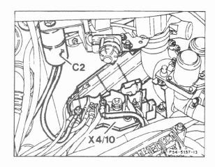
C2 Electrolytic capacitor (alternator/battery harness noise suppressor)
