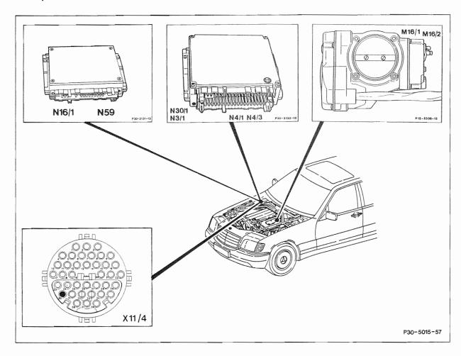
M16/1 Electronic accelerator actuator
