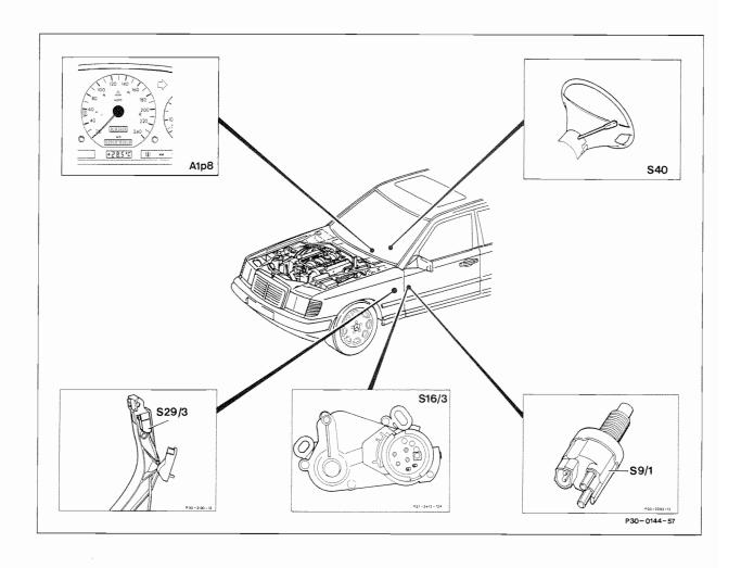
A1p8 Electronic speedometer S40 Cruise control switch
