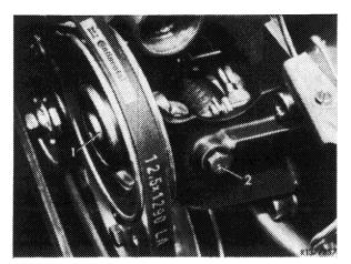
Guide pulley on cylinder head engine 110
