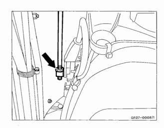
2 Turn lock (40) upward in direction of arrow.
