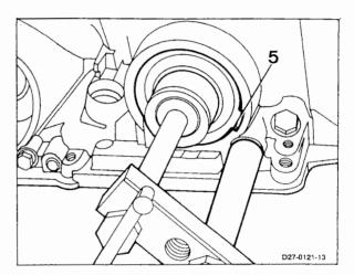
**85** Screw hexagon bolt into tester by hand until a resistance becomes noticeable.
