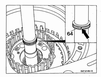
28 Engage assembly lock (arrow) on brake band B1 (56).
