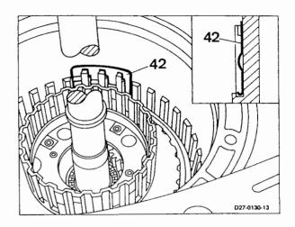
79 Remove and disassemble clutch K2 (49), refer to 5.4/1.
