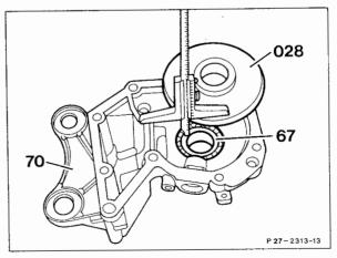
67 Dimension "a" minus dimension "b" = axial clearance "C". The axial clearance "C" must be 0,4 to 0,5 mm.
