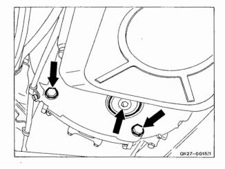
**18** Put down transmission in upright position and remove torque converter.
