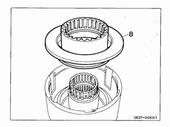
8 Remove lip sealing rings (9/10) of piston.
