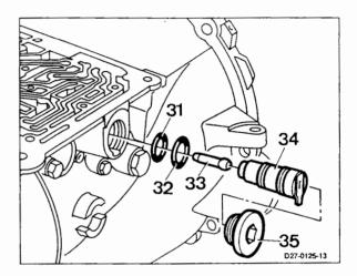
34 Insert O-ring (6) and brake band guide B1 (15), make sure that the fixing stud engages in the bores in the housing and press in until they noticeably engage.
