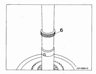
3 Remove snap ring (1) with screwdriver.
