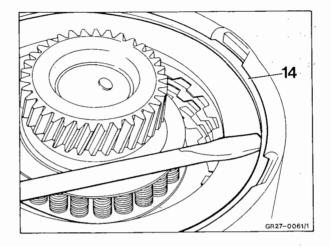
**14** Measure clearance "A" using a feeler gauge. The disk clearance must be 0,7 up to 1,3 mm.
