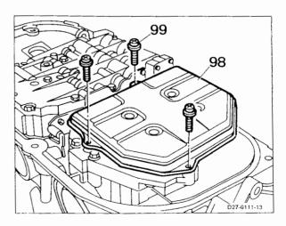
**126** Mount oil pan (105) with new seal (103) and tighten hexagon bolts (104) to specified tightening torque.
