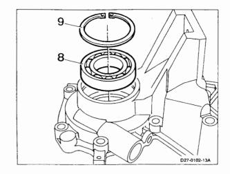
3 Measure clearance between locking ring (9) and ball bearing (8) with feeler gauge.
