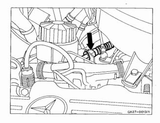
**14** Detach end cover from torque converter housing.
