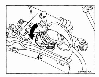
9 Engage control rod and install retainer.
