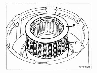
**6** Mount assembling fixture, press down spring retainer and remove snap ring (5).
