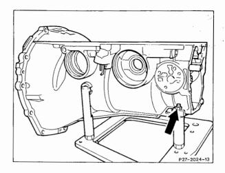
2 Insert plastic guide ring (22) for piston B2, then insert lip sealing ring (23) with the shop-made drive-in drift.
