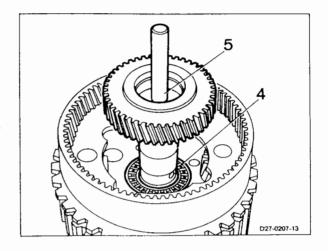
17 Install front planetary gearset (3) with input shaft.
