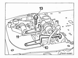
119 Mount shift valve housing (100) and tighten hexagon bolts (100/102) to 8 Nm.
