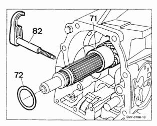
27 Remove locking ring (71) with pair of pliers.
