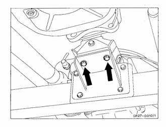
11 Mark installation position of propeller shaft, detach and tie up to the side.
