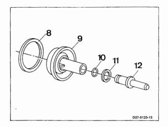
**Note:** from July 1990 to September 1990 (transmission no. from 03 420 691 to 03 450 408) the brake band piston B1 was installed with an automatic adjustment of the loose play. The loose play therefore does not have to be measured or adjusted in these transmissions. Standard as from 8.92.
