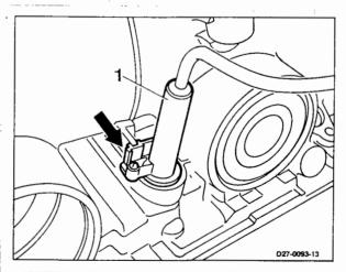
130 Insert thrust pin (3), spring (2) and modulating pressure valve (1).
