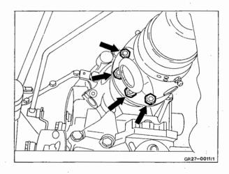
**6** Unscrew twelve-point collar nut (14) and remove flange (13).
