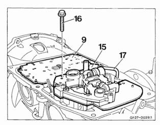
**Note:** Prior to tightening the lower cover, make sure that the oil pipe (17) is inserted in the bore (arrow) free of tension.
