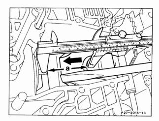
**103** Press brake band **B2** at the support strap to pressure body (direction of arrow) and measure dimension "b".
