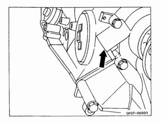
76 Install kick-down solenoid valve (75) with solenoid (76) and new gasket (77) and tighten to 30 Nm.
