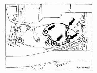
15 Detach torque converter from driver.
