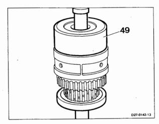
18 Insert gearset in transmission housing, at the same time turn the input shaft (87).
