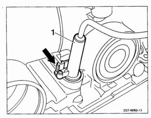
5 Disengage pull rod (arrow) and remove O-ring (2).
