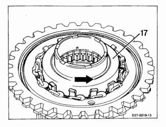
**5** Insert new O-ring (16) and mount support disk (15) in such a way that the journal (arrow) engages in the bore (arrow) in the free wheel outer ring.
