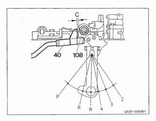
**Note:** The clearance "C" is adjusted by changing the plastic clip (109).
