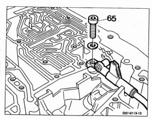
**52** Pull out range selector shaft (30) and remove detent plate with linkage (40).
