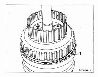
Lift front planetary gearset (3) with input shaft.
