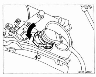
9 Engage control rod and install retainer.
