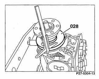
66 Place graduated disk (028) on sealing surface of rear cover. Using the depth gauge, measure from the graduated disk (028) to the inner race of ball bearing (67).
