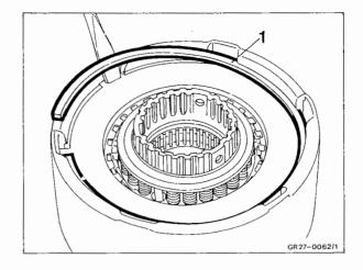
3 Remove complete disk set from the outer disk carrier (11).
