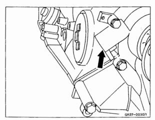
10 Unscrew twelve-point collar nut (96) and remove flange (95).
