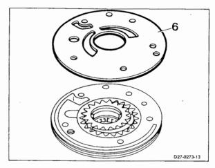
**6** Insert primary pump in front transmission cover (8) and tighten hexagon bolts (11) to 20 Nm.
