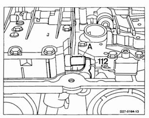
**Note:** The range selector lever (113) must engage in the follower (arrow) of the detent plate.
