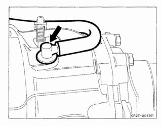
**134** Remove bolt (arrow) and lift transmission out of assembly block.
