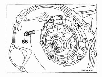
73 Screw bolts into the threaded bores and in this way pull out front transmission cover (110) with sealing ring and disassemble, refer to 5.2/1.
