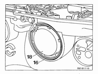
Measure free travel at brake band B2 and adjust
