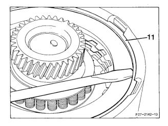
3 Remove complete disk set (15) from outer disk carrier.
