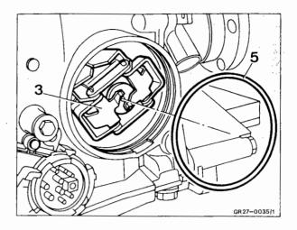
**48** Swivel axial support to flyweight governor so that it engages in the groove in the governor shaft
