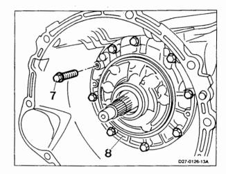
4 Screw bolts into threaded bores and in this way pull out the front transmission cover (8) with seal.
