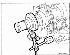
**Note:** Once the dimension of 0,07 mm is exceeded, detach the flange. Turn the flange and install again.
