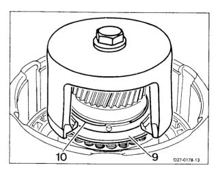
**6** Remove spring retainer (9) and pressure springs (8).
