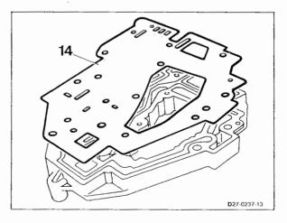
109 Mount seal (8) and intermediate plate (9) on lower cover.
