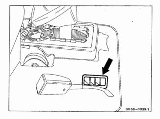
10 Make a cut of approx. 4 cm in the left and right of the carpeting, at the rear edges of the tray.
