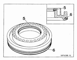
5 Insert installation sleeves in the outer disk carrier.
