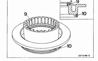
2 Insert installation sleeve in the outer disk carrier.
