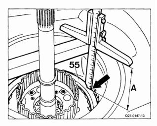
Note: Reinstall cup spring and steel disk in the correct order after measurement.
