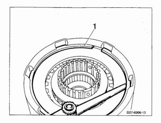
**Note:** The disk clearance is adjusted by changing the snap ring (1).
