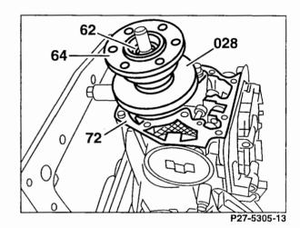
.65 Using the depth gauge, measure from the graduated disk (028) to the seal.
