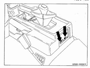
**9** Disengage tensioning rubber piece for belt whip and detach left and right nozzles.
