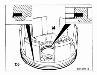
8 Oil the sliding surfaces of the installation sleeve and mount on the front transmission cover (8) (arrow).
