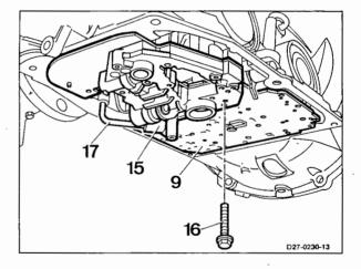
**Note:** Before tightening the lower cover, make sure that the oil pipe (17) is inserted in the bore (arrow), free of tension.
