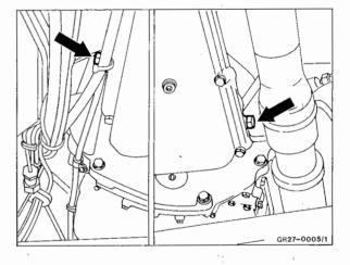
5 Remove plug connector for starter lock switch.
