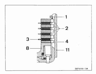
9 Insert complete disk set in the outer disk carrier (11).
