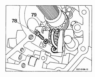
20 Release lock nut (106 or 44) and move axial support (82) away from the flyweight governor (107) using a screwdriver. (direction of arrow)
