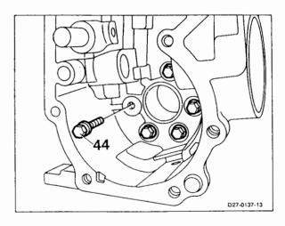
7 Screw in bolts (44) and tighten to 11 Nm.
