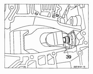
**81** Clamp together brake band B2 (48), position horizontally and remove.
