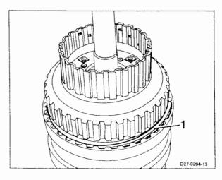
**19** Install lubricating pressure ring (6) in the input shaft.
