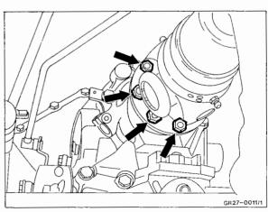
8 Screw in drain plug (35) with new sealing ring (36) and tighten to 14 Nm.
