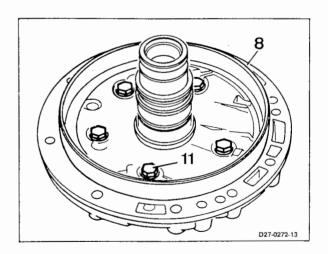
7 Check lip sealing rings (13/14) and replace if necessary.
