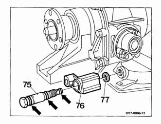
9 Check dummy plug, replace if necessary.
