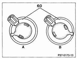
A Basic adjustmentB reduced by 0,2 bar
