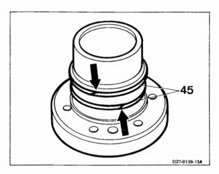
**6** Center supporting flange (46) with two hexagon bolts, approx. 80 mm in length, to the hole pattern of the fastening bores and drive in.
