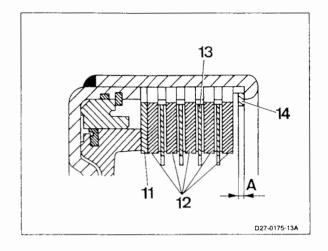
12 Insert disk set (15) in the outer disk carrier.
