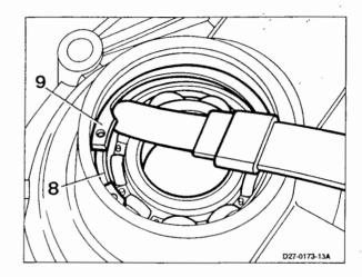
4 Drive in new radial shaft seal to be flush using a suitable drift.
