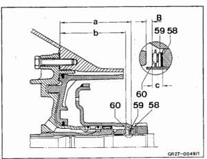
40 Insert Teflon rings (9) with grease.
