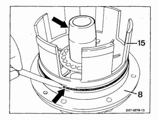
**Note:** Insert piston LB3 (15) in such a way that the journal (arrow) on piston LB3 coincides with the bore on the front transmission cover.
