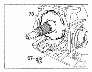
17 In vehicles with electronic speedometer, from transmission end no. 37 47 000 remove parking lock gear (73) with rotor, parking lock ratchet (74) and expanding spring (75).
