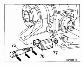
77 Preassemble brake band piston B1 (9). For this purpose insert shim rings (11) and new sealing ring (10).
