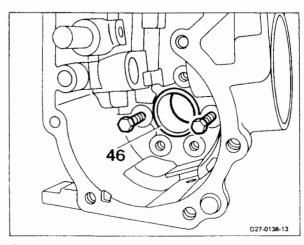
8 Insert support disk (47) in such a way that the strap for the anti-torsion device is in the corresponding bore (arrow).
