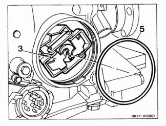
**3** Turn axial support at slot (A) in clockwise direction (direction of arrow) up to stop.
