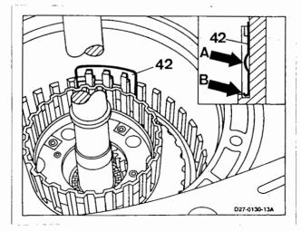
22 Put together disks for the brake B3 in the following order and insert individually.
