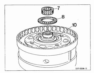
9 Remove radial bearing (9) from output shaft.
