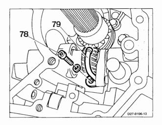
**57** Slide roller (81) on linkage (40) of detent plate and insert plastic guide (80) in housing.
