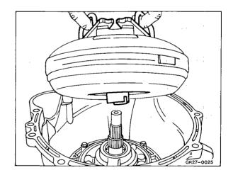
2 Check projection (K) towards torque converter housing.
