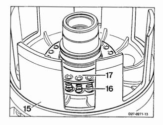
14 Place spring tensioner on spring retainer (17) and clamp with counterpiece until the groove for the snap ring (18) is exposed.
