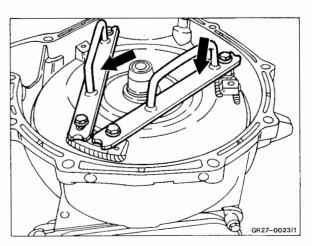
19 Flush torque converter, for this purpose fill with 1 liter of petroleum. Insert flushing drift (063) and drive with a hand drilling machine at reduced speed for approx. 2 minutes. Afterwards drain petroleum via the drain plug.
