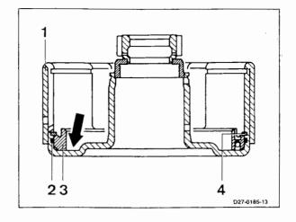
4 Oil lip sealing rings (5/6) with ATF oil and insert in annular groove of the piston with the sealing lips pointing down.
