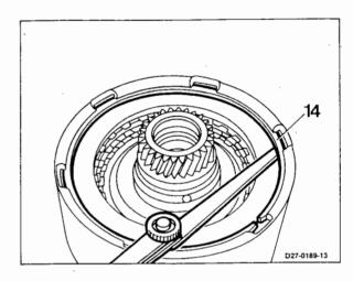
**Note:** The disk clearance is adjusted by changing the snap ring (14).
